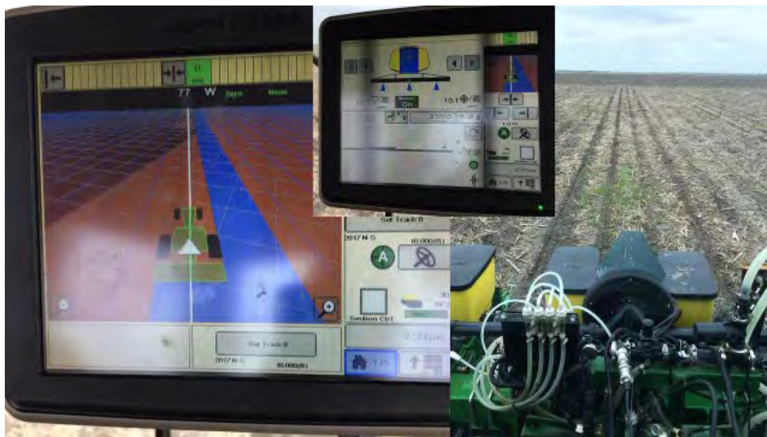
Figure 4. Variable rate liquid application system for applying fertilizer during planting.
